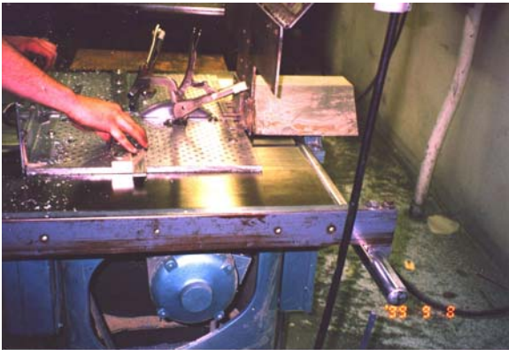
This is the saw set up used to cut the aluminum and copper
