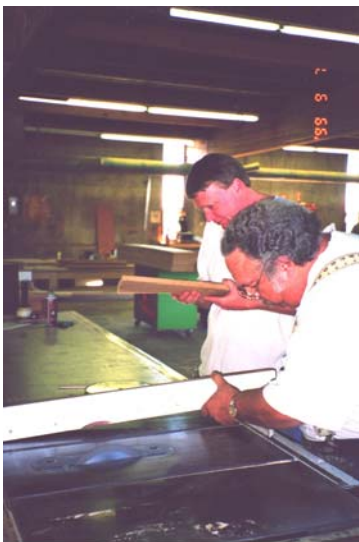
This is a hard laminate on a soft core. It is very difficult to cut without chipping or blow
