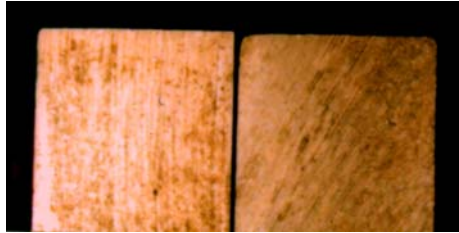
Two pieces of copper – left one cut with a carbide tipped blade and right one cut with a ceramic tipped blade
