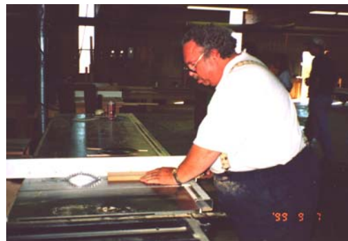
This is a hard laminate on a soft core. It is very difficult to cut without chipping or blow
