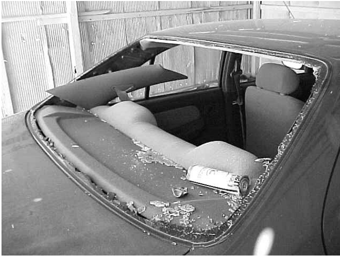
Spray can in hot car – blew up and blew out rear window
