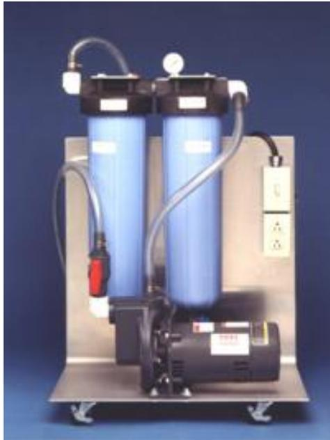
We now have a filter system that filters straight oil coolants. Above is our CP 2020 which filters tight oil coolant very well. It is also available as a wall mount unit.
