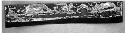
Untreated – patchy silver solder adhesion
