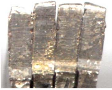
This is a 4x photo of four failed tips. You can see the grind marks on the steel in all four tips. You can also feel the grind marks by dragging your thumbnail over them. The grind marks can even be seen faintly with the naked eye in some places
