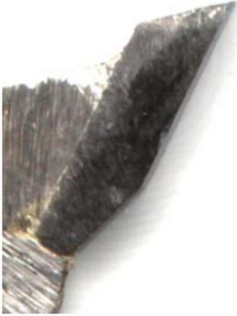
Above is a photo of a tip on the same saw. This tip did not come off. We ground the tip and carbide to expose the braze joint. There is very little braze alloy between the steel and the tip
