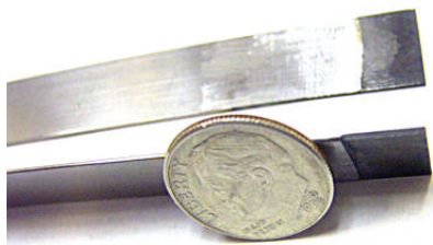
Carbide butt brazed to steel shown resting on a dime.
