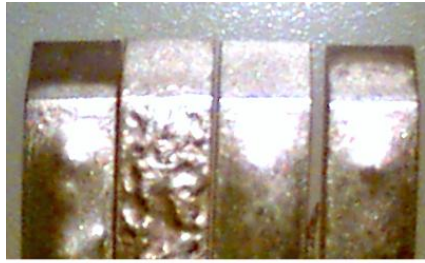
Overcooked and burnt tips Braze alloy on the face
