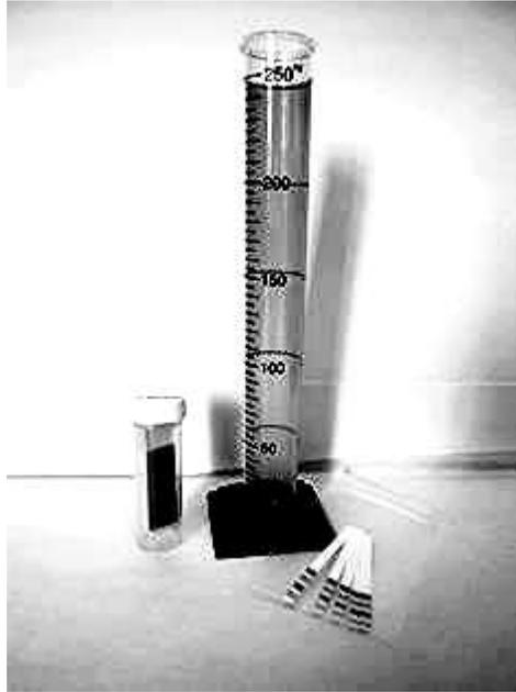
A Free kit for testing your Machine Coolant.
