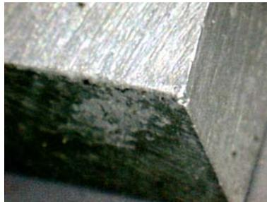
This is the tip after 100 passes on each of the three sides shown. The light patch in the dark area is a dip in the surface that I didn't get down to.
