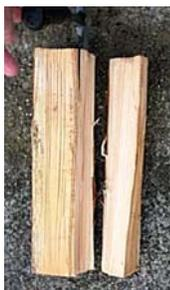
When you cut wood down the grain it is much easier to separate it in smaller pieces than it is cutting across the grain.
