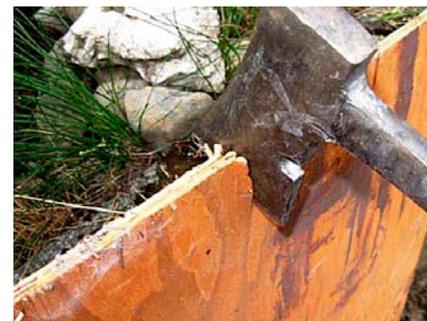
When you hit piece of plywood you can initiate a crack but it doesn't go anywhere. You have to keep cutting and cutting in the same place until you gnaw your way through it.
