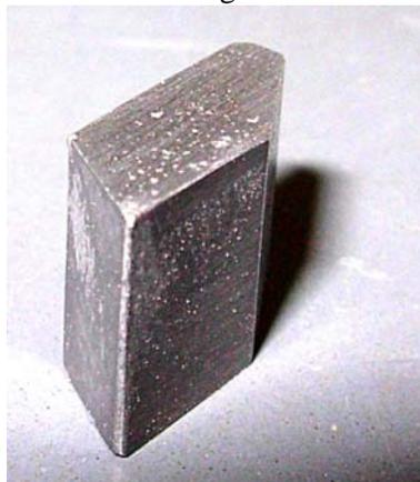
As near as I can tell you would need about 500 to 1,000 passes with a coarse hone to "sharpen" this tip. 500 passes would be about two and a half minutes. The four sides of a saw tip would mean about ten minutes per tip. You could sharpen a 24 tooth saw blade in just four hours with a coarse diamond hone.
