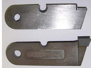
Top is an inserted tooth machined out of a solid steel billet. Bottom is a traditional cast part. The solid steel, machined part is much tougher, lasts longer and is much tougher.
