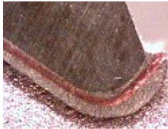
Here you see that the braze alloy was heated enough to soften it but not enough to achieve full flow. The amount of alloy between the tip and the copper is about right. There is appears to be more alloy between the copper and the steel because this alloy was squeezed out leaving a thin joint.
